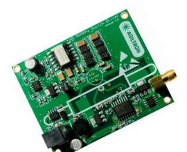
The NSDR series of drivers provide high voltage of signals to drive the NS and NP as well as NF series of solid state switches. The push-pull output design ensures fast transition for both rising and falling edges with the high repeat rate, and it is especially suitable for driving capacitive switch loads.
